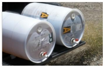
EFS drum set, using PVC ball valves, with "R" and "A" clearly labeled.
